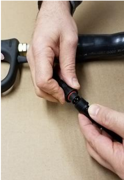
Connect 3-Pin electrical connection between Hose and Dispensing Gun
